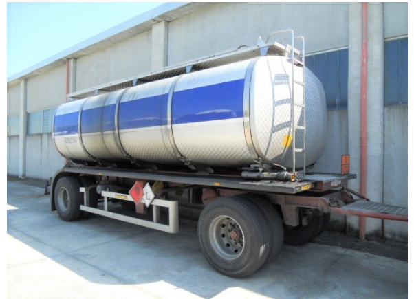
2 axles trailer, pneumatic suspension 22-AB611 with ABS, drum brakes
