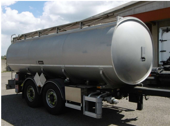
2 axles trailer, pneumatic suspension 22-AH008 with ABS, disk brakes
