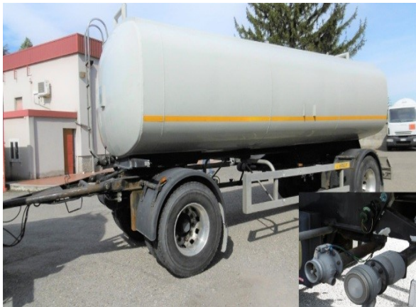
2 axles trailer, pneumatic suspension 22-VA023 with ABS, drum brakes
